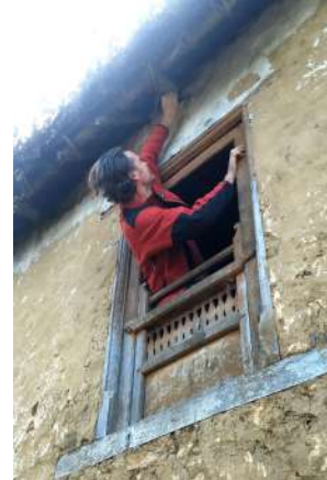
Left : The house with thatched roof selected for the thermal behavior experiment, at Mathillo Suping, 1.500m. Right : Carles Turró setting up the outside temperature sensor under the roof's eave.
