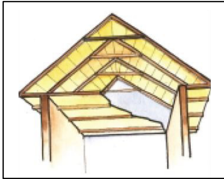
Roof truss with collar beam (horizontal tie)
