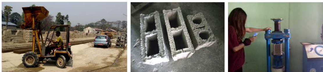
Manufacture of "Awasuka blocks" and load-bearing tests by comparing local blocks to Awaskua blocs.
