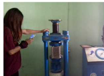
Manufacturing of "Awaskua blocks" and load-bearing capacity tests, comparing local blocks to Awaskua blocks.
